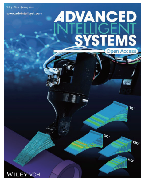
Figure 1: Among other crossbeam angles, the Fin Ray model with nonstandard 10°-inclined crossbeams has a greater contact area to a curved surface and better durability. It can enhance the efficiency of on-pipe robot locomotion. The work has been chosen for the front page of Advanced Intelligent Systems.
