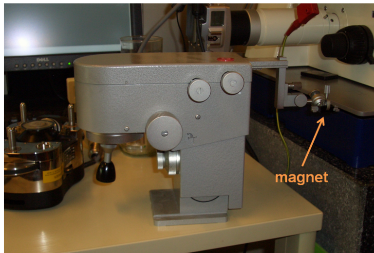
Figure 93: A permanent magnet mounted on a precision lever allows for reproducible tip magnetization.
