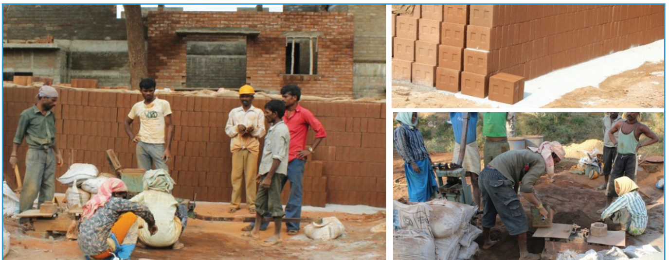
Figure 15 SSB block production teams and stack of SSBs
