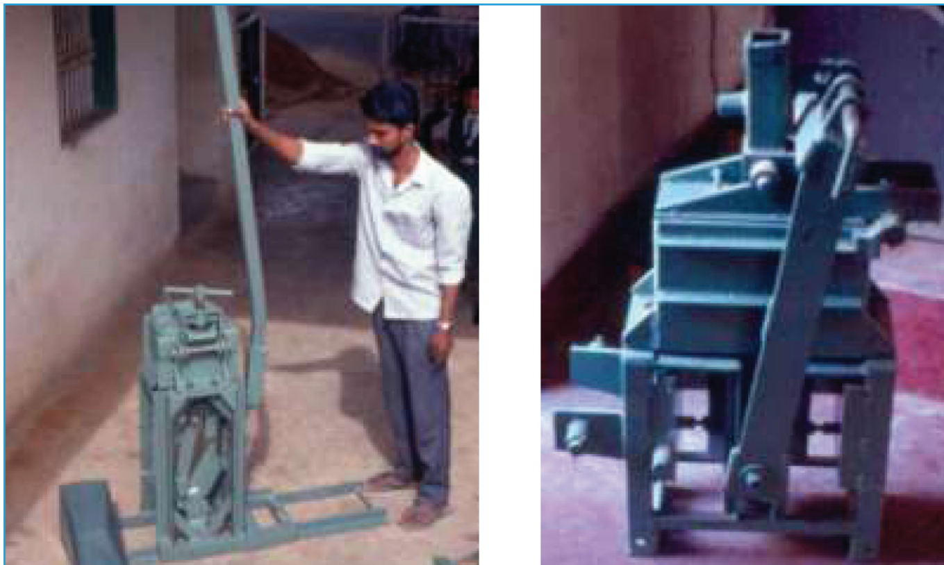
Figure 6 The toggle press (L) and the reverse toggle press (R)
