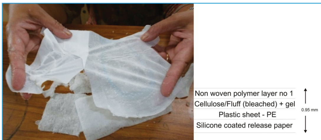
Figure 5 Layers in a pad
