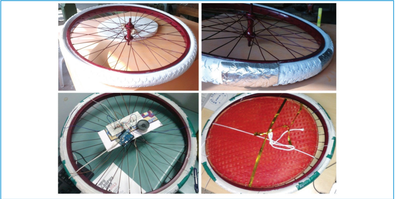
Figure 2 Round piano prototype with an Arduino board mounted at the centre in order to allow the rotation of the wheel with touch-sensitive aluminium foil on the sides
