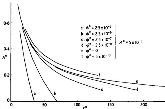
Fig. 3. Theoretical variation of film thickness with time for porous elastic layers
