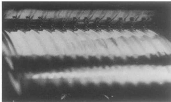
(f) Rippled surface layer of oil emerging from cavitating region on rotating cylinder near a plane
