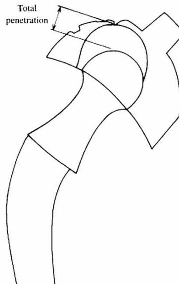
Fig. 10 Worn Charnley hip joint (PTFE)
