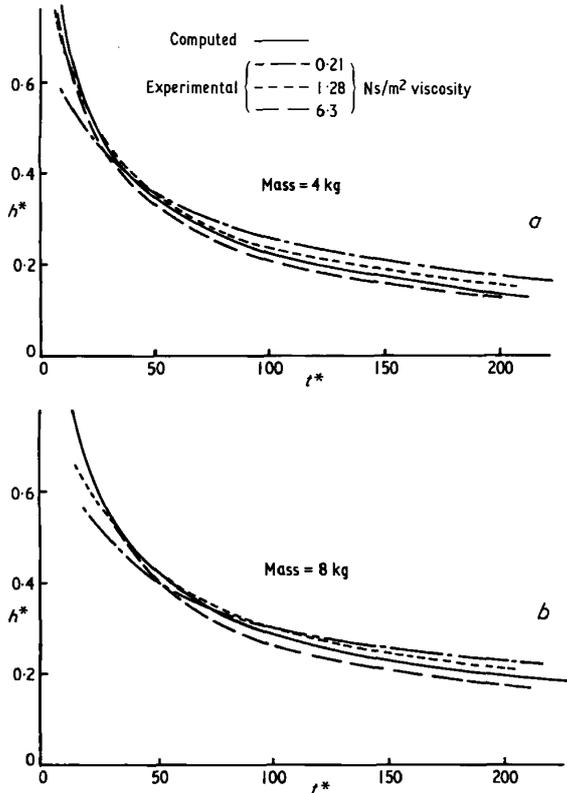
Fig. 8. Experimental and theoretical film thickness/time characteristics for the perforated layer
