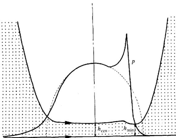
Fig. 7 Essential features of elastohydrodynamic line contacts
