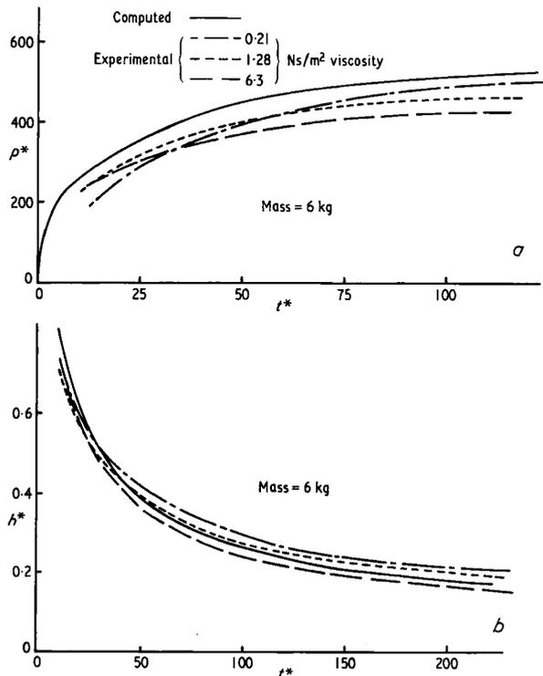
Fig. 7. Experimental and theoretical pressure and film thickness/time characteristics for the perforated layer
