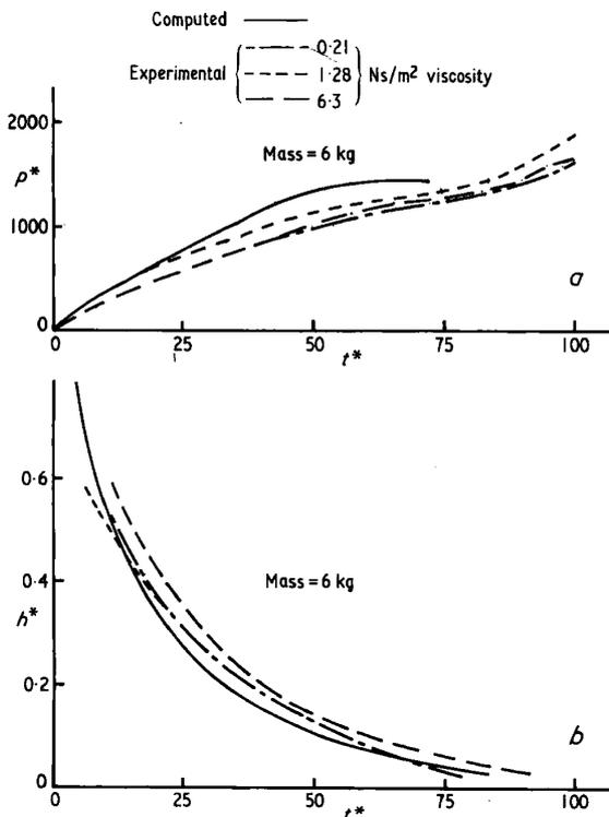
Fig. 5. Experimental and theoretical pressure and film thickness/time characteristics for the low-permeability flexible layer
