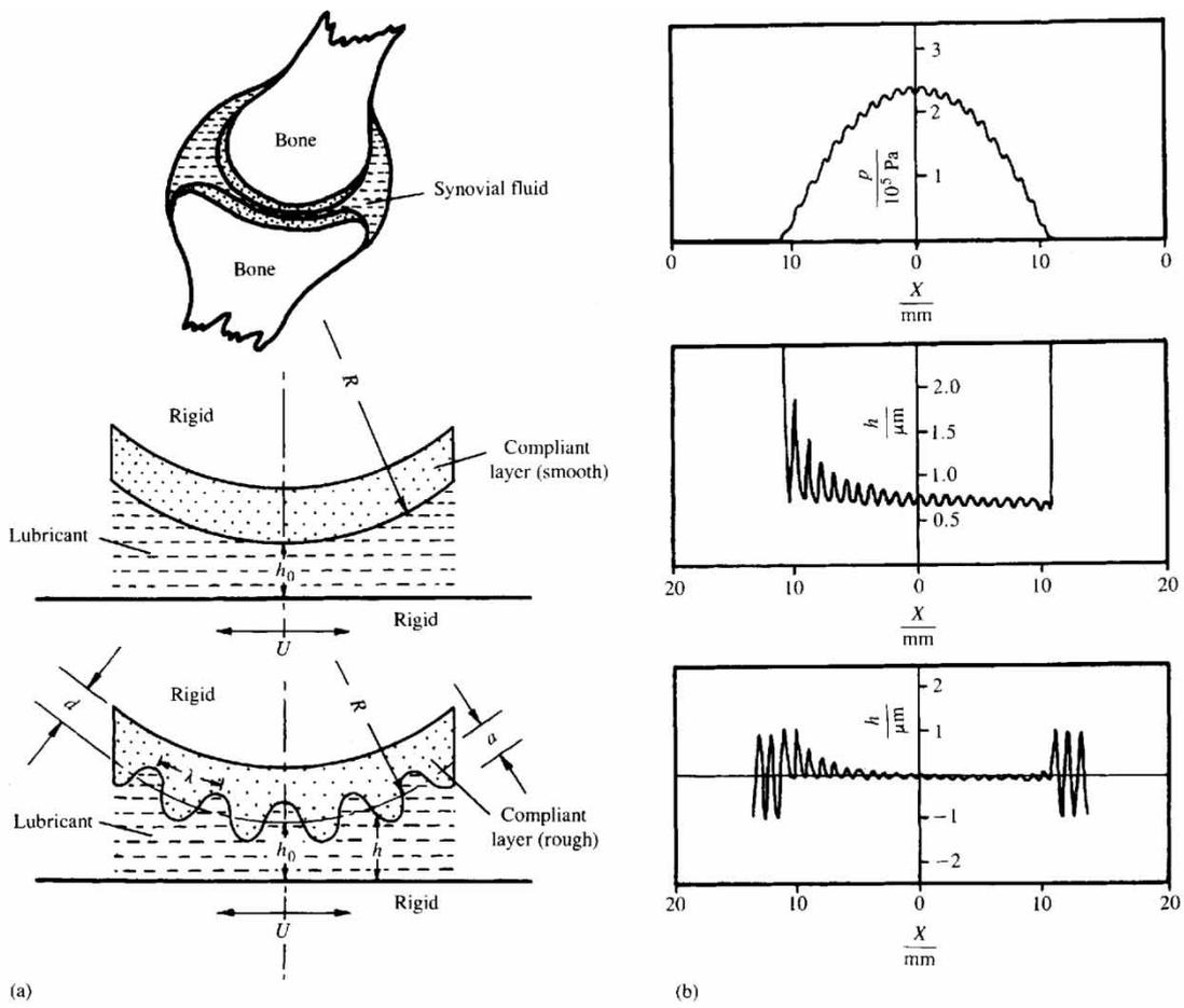
Fig. 9 Micro-elastohydrodynamic lubrication in synovial joints
