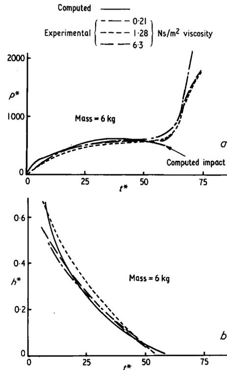
Fig. 6. Experimental and theoretical pressure and film thickness/time characteristics for the high-permeability flexible layer
