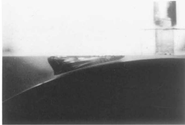
(b) Rotating cylinder near a plane (side view)
