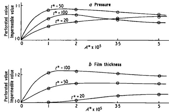
Fig. 4. Comparison of theoretical centre-line pressures and film thicknesses for the perforated layer and the impermeable layers
