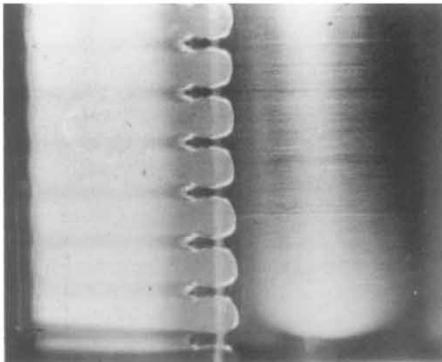
(e) Oil streamers penetrating into air bubbles in the cavitating zone between a rotating cylinder near a plane
