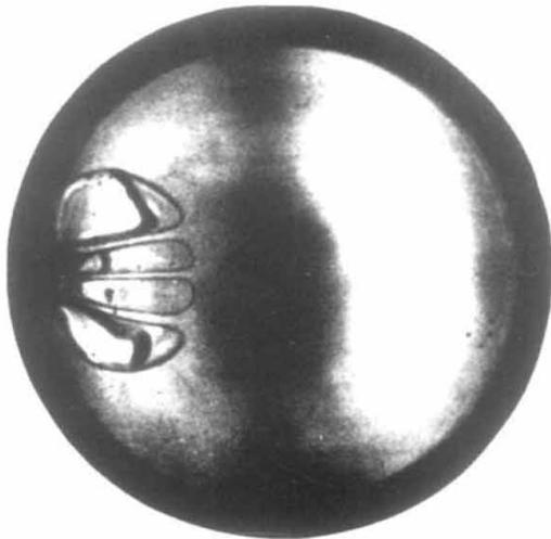
(c) Glass lens near a moving metal plate (steadily loaded)
