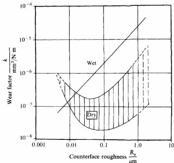
**Fig. 11** Influence of environment and stainless steel counterface roughness on the wear of ultra-high molecular weight polyethylene (UHMWPE)
