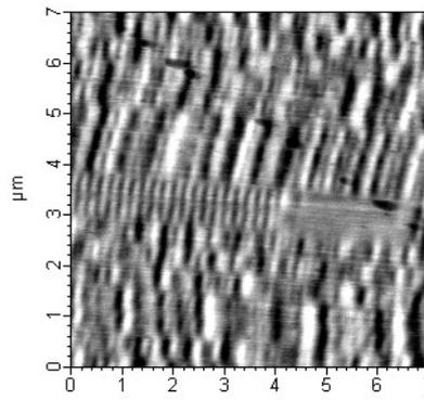
figure 6: 2 GB hard disk  $\mu\text{m}$
