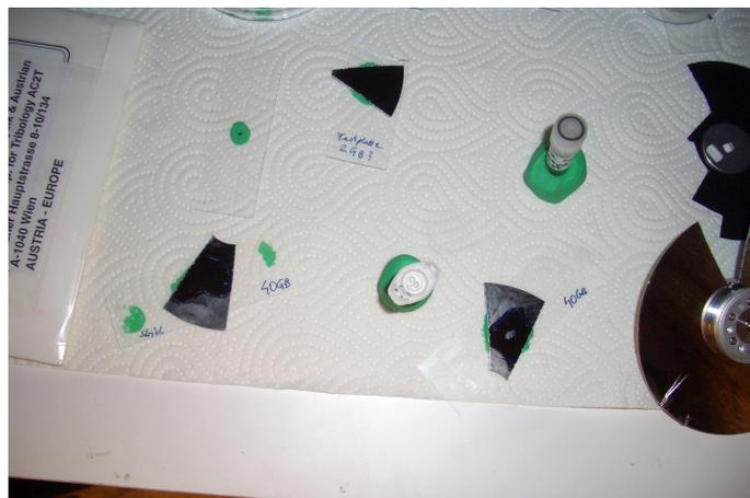
*figure 1: 40 GB sample for MFM measurements*
