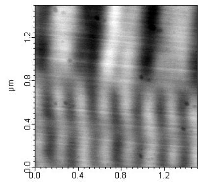
figure 7: 2 GB hard disk detail scan  $\mu\text{m}$
