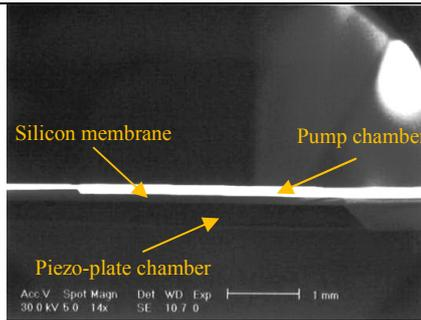
Fig. 7. Cross-section view of fabricated membrane after double sided silicon etching
