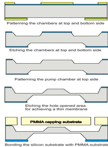
Fig. 2. Schematic fabrication process of valveless micropump using double-sided etching
