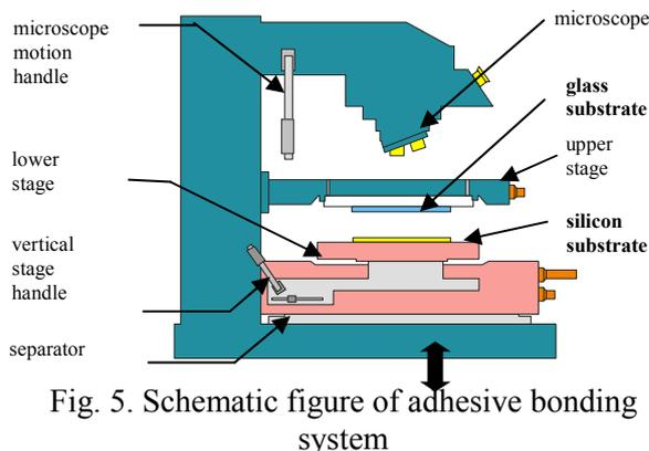
Fig. 5. Schematic figure of adhesive bonding system
