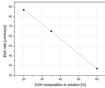
Fig. 3. Etch rate profile of KOH solution for <100> silicon
