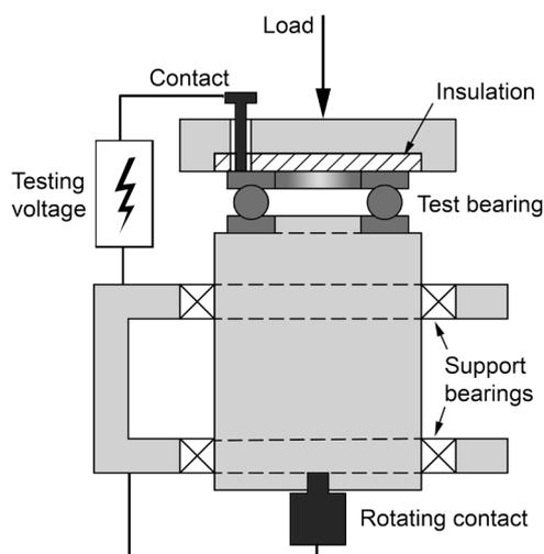
Figure 3: Sketch of the test rig's mechanical set-up
