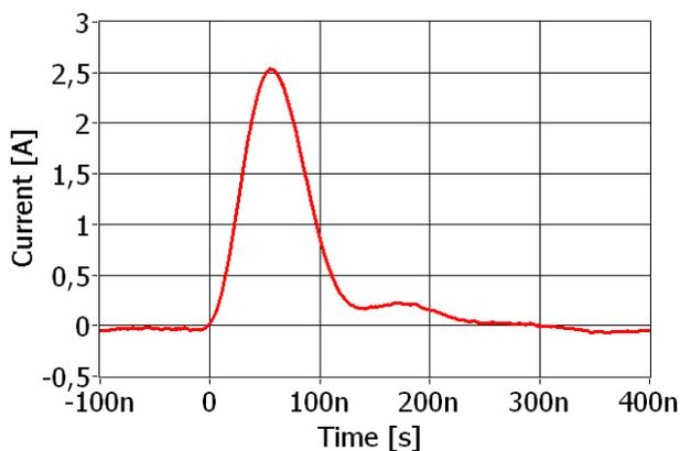
*Figure 5a: Current pulse with short-circuited terminals with  $V_d = 30V$*
