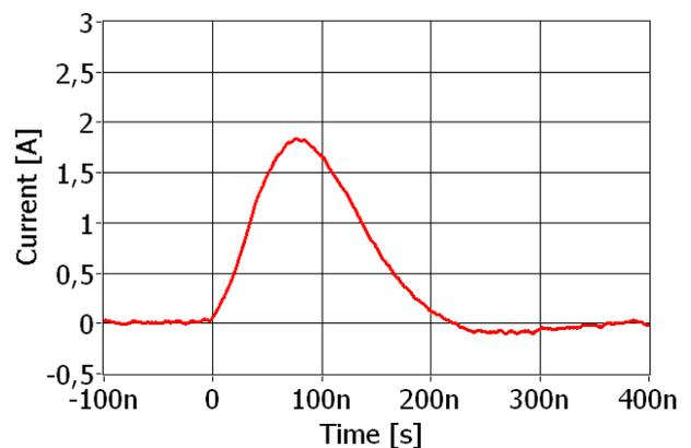
*Figure 5b: Current pulse applied to bearing at 1000 rpm with  $V_d = 30V$*
