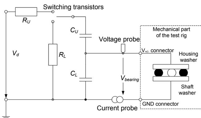
*Figure 4: Operating principle of current-applying electronics*
