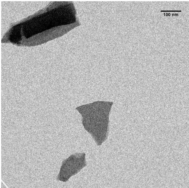
*Fig. 7: Some HOPG flakes produced with method 3.*
