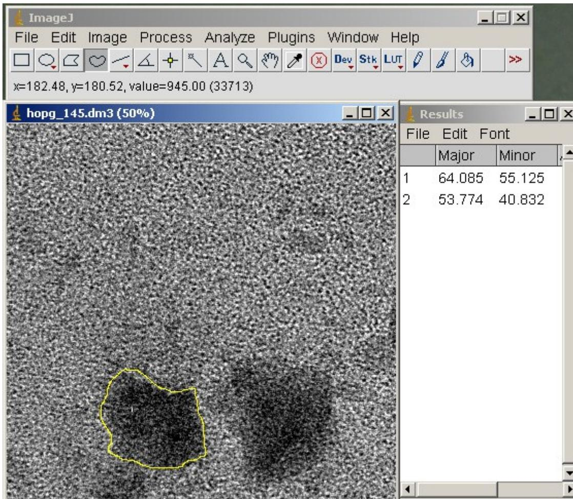
Fig. 11: Determination of particle size with ImageJ. Yellow: currently selected particle.
