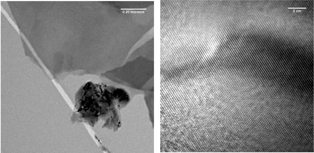
*Fig. 8a: On places like this, where the SiO coat was ripped by accident (diagonal bright line), high resolution could be achieved over that cleft.*
