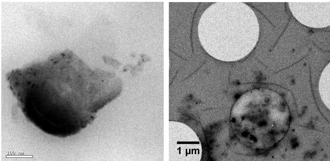
*Fig.5a: HOPG nanoflakes prepared with method 1 (scotch tape).*
