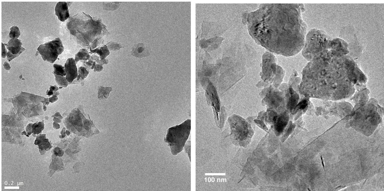
*Fig. 10a,b: Two different particle types can be recognized. The rounded, dark things are Si. The flat, layered particles are graphite.*
