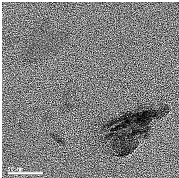
*Fig. 6a: Particles prepared with method 2. On the smaller particle on the right side, faint lines are visible, probably rows of atoms.*
