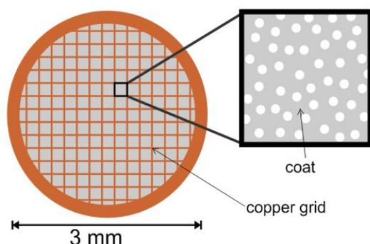
*Fig. 3: TEM grid with holed coating*
