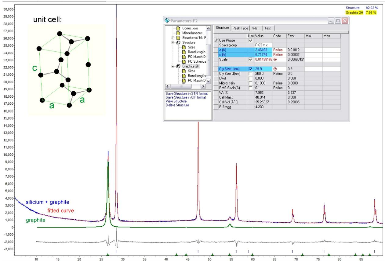
Fig.12: Fitting a curve to the powder diffraction measurement result.
