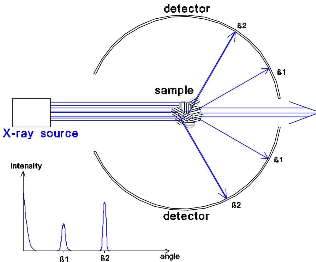
Fig. 4: Schematic X-ray powder diffractometer
