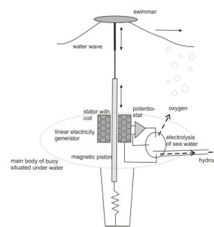
Figure 3: Schematic of a possible buoy design. To allow for a cheap modular installation and easy maintenance, the design should be kept as simple as possible. (Tributsch 2012)
