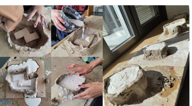
The third task involves creating a negative of the clay form using casting gypsum. The students build a water-tight clay wall around the form, leaving a one cm gap for plaster pouring.
