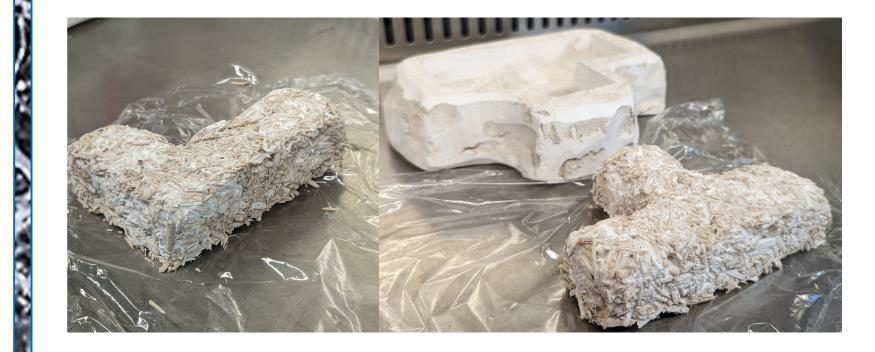
The mycelium filled Negatives of all participants are now left to incubate for one week at an incubation temperature of around 24 degrees centigrade (next to the clay oven) and a high humidity (an open water container will be placed in the incubation tent). Five days normally suffice for incubation of the mycelium, but that would not fit the student's schedule. It will be arranged for the students interested to visit the incubation tent halfway through the week.
