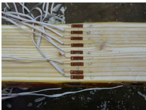
Fig. 1a Poplar board with 9 strain gauges
