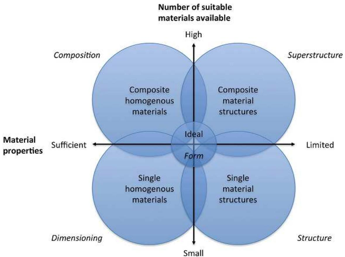
**Figure 10: Structuring facilitates more complex functionalities.** Current MEMS are mostly relying on the properties of single material structures. Since this approach limits the complexity of functions that MEMS, consisting of few elements, structuring the materials can replace the common technological approach of adding more, different materials to accommodate increased functionality. © by (Gebeshuber & Gordon, 2011)
