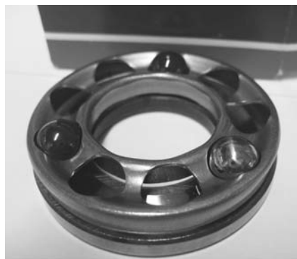
Figure 2: Test bearing consisting of one steel test RE and two ceramic supporting RE
