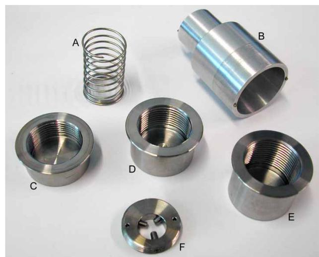
**Fig. 4** Modified AFM closed fluid cell for tribological investigations of large samples in chemically aggressive environments. (A) Stiff spring, (B) spanner, (C), (D), and (E) container pots, and (F) sample holder
