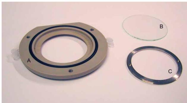
**Fig. 1** Lower part of the conventional closed fluid cell supplied with the MFP-3D. (A) Base with plugged Luer fittings, (B) glass disc sample holder, and (C) ring for fixing the glass to the base
